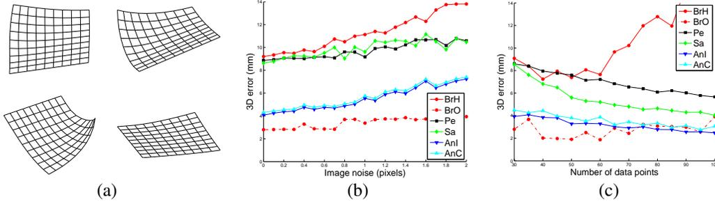
Figure 2. **Results on synthetic datasets.** (a) Examples of simulated developable shapes. (b) 3D reconstruction error against image noise. (c) 3D reconstruction error against number of data points. **BrO** is a non-convex and non-analytical method that serves as gold standard. the proposed analytical methods **AnI** and **AnC** thus give more accurate results than existing convex methods.
