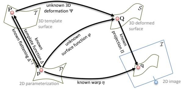
Figure 1. **General modeling of monocular template-based reconstruction.** The surface is assumed to have a disk topology.
